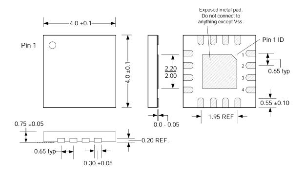
Note: All dimensions in <u>millimeters</u>. Care must be taken to ensure PCB traces and vias are not placed within the exposed metal pad area.
